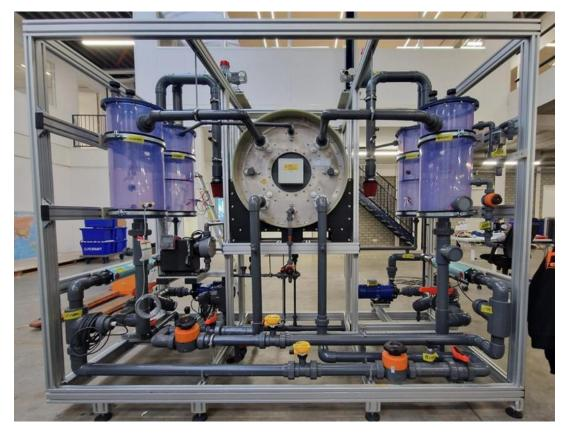
The results are good at 100% N-removal at a total energy use < 7 kWh/kg N removed, the target number. The concentration of NH3 that comes out of the process is 10%.
